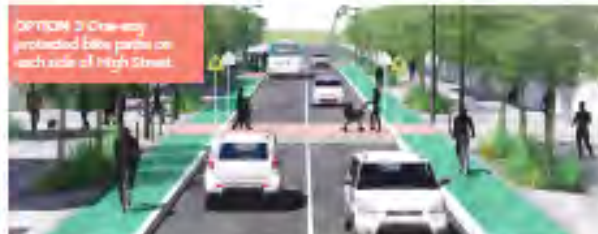
OPTION 3 One-way protected bike paths on each side of High Street. Bikes and cars are separated. There are protected bike lanes on both sides of street, on-street parking is removed, there are wider footpaths and there is potential to double the number of street trees.
