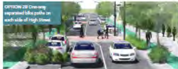
OPTION 2B One-way separated bike paths on each side of High Street. Bikes and cars are separated. One-way bike lanes form part of footpaths on both sides, there is reduced on-street car parking staggered across both sides, and there is potential to double the number of street trees.
