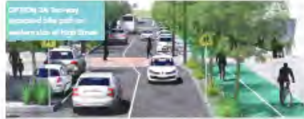
OPTION 2A Two-way protected bike path on western side of High Street. Bikes and cars are separated. Two-way bike lane forms part of the footpath on the western side, there is reduced on-street car parking staggered across both sides, and there is potential to double the number of street trees.
