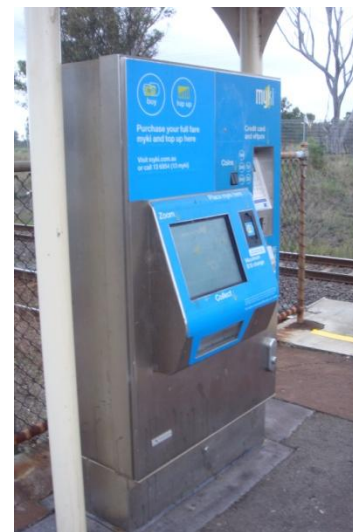
Lack of appropriate supports at fare payment point
