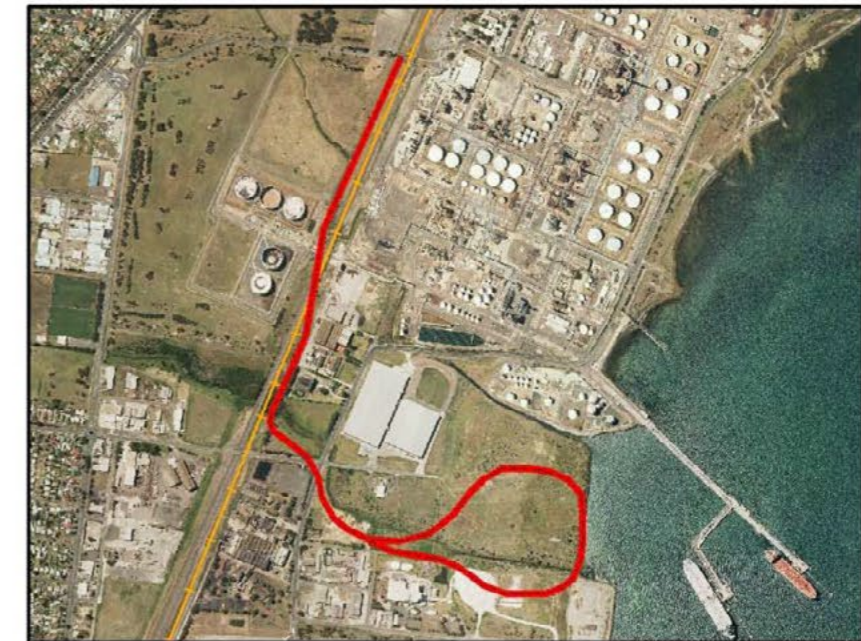
(5g) New rail loop to service Lascelles wharf. Bridge crossing required across existing mainline.
