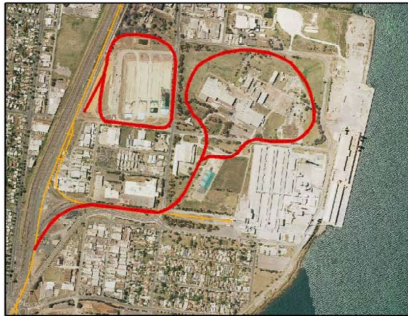
(5c) Rail loop to 'One Steel' to service Lascelles or a loop to the Graincorp bunker site. (As contemplated by Fig 5a)
