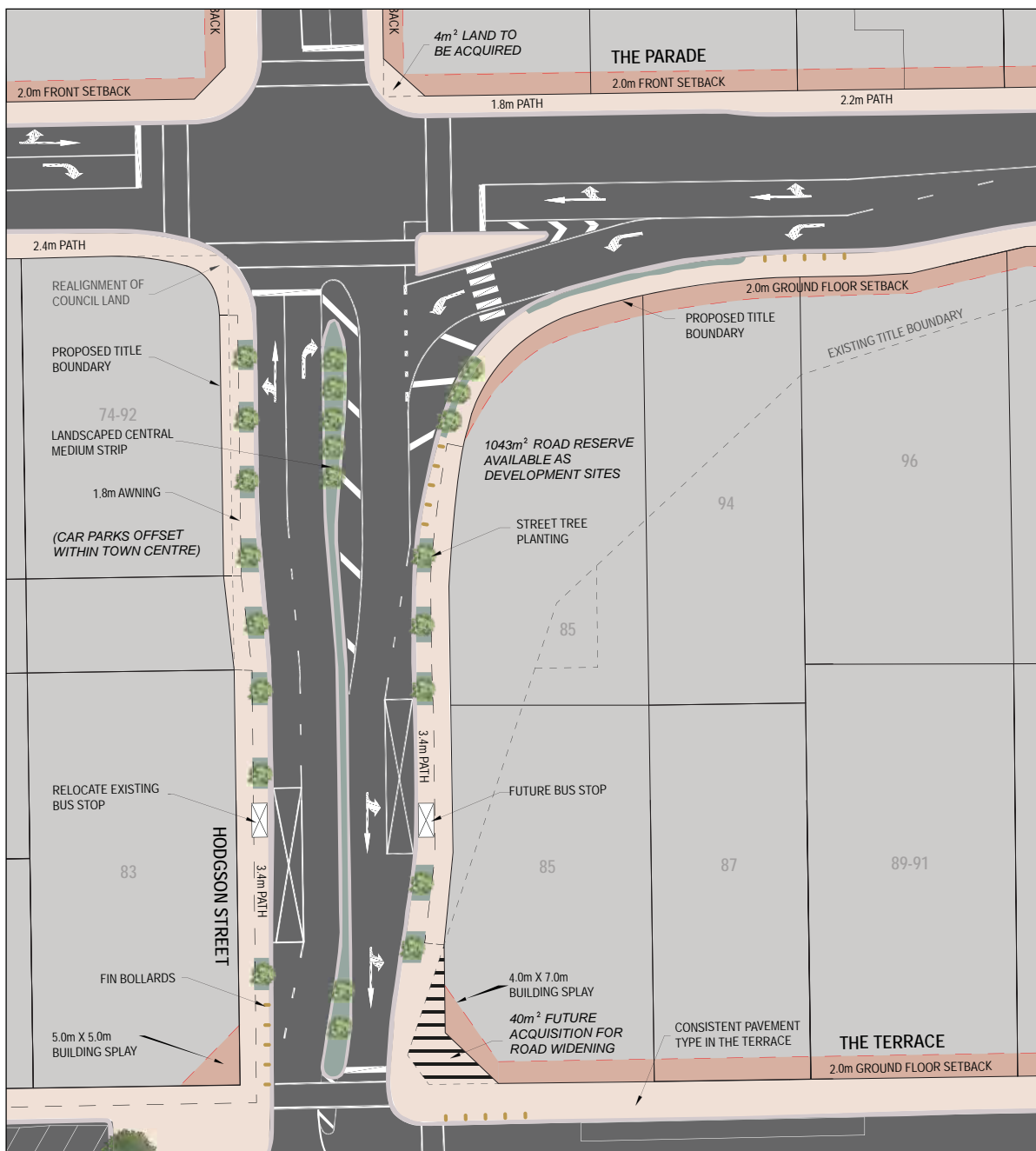
Figure 35: Hodgson Street streetscape upgrade concept plan showing the street layout using signals
