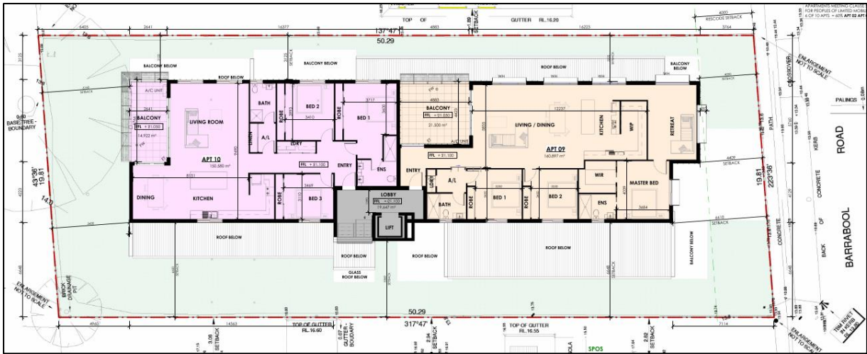
Figure 16: Upper (second) floor plan showing common area entry, apartment and private open space (balcony) layouts. Source: Application documents.
