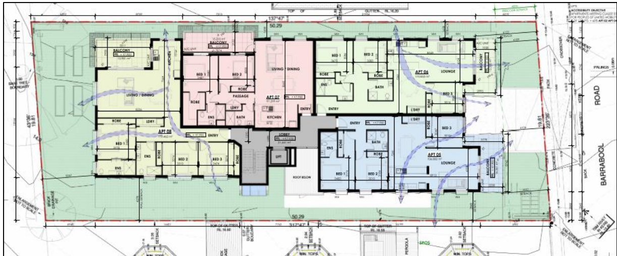
Figure 15: Mid (first) floor plan showing common area entry, apartment and private open space (balcony) layouts. Source: Application documents.
