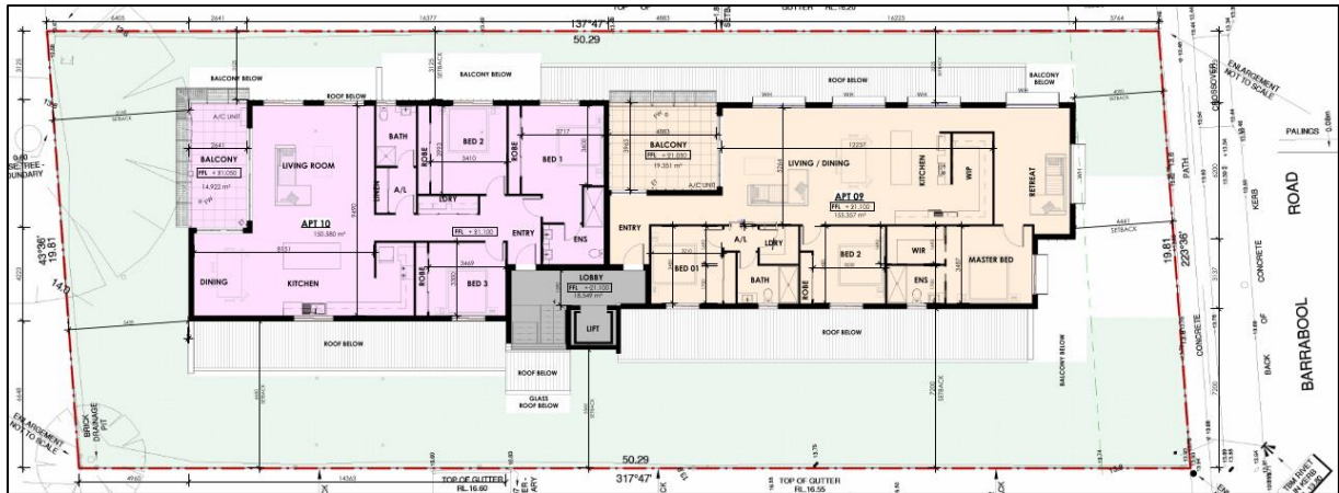
Figure 16: Upper (second) floor plan showing common area entry, apartment and private open space (balcony) layouts. Source: Application documents.
