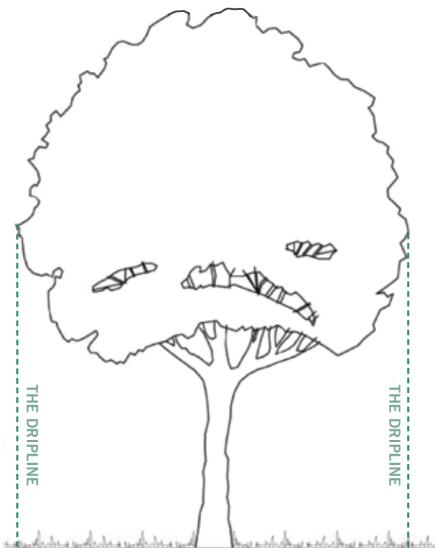
FIGURE 6: Tree Protection Zone - Dripline
