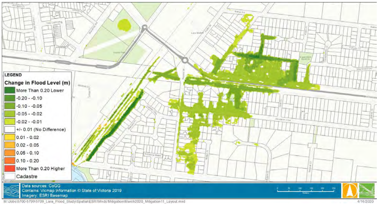
Figure 4 Kyema Drive & Clover Street Pumping Difference Plot (Mitigation Minus Existing)
