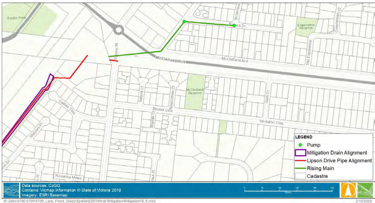
Figure 3 Kyema Drive & Clover Street Pumping Layout
