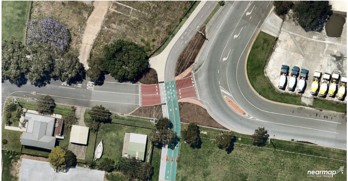
■ Figure 5.2: Example of path priority crossing with the ramps ahead of the crossing (Somerset Street / McDonald Road, Windsor Queensland)
