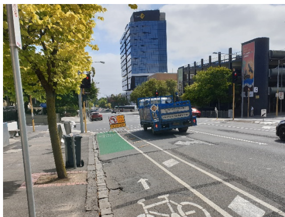
(c) Northbound approach to Little Malop Street (note roadworks sign impeding bicycle lane)
