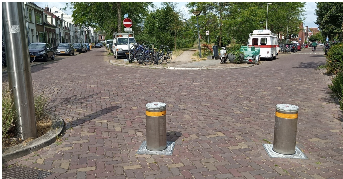
Figure 7 Local traffic only: Using automatic bollards to restrict car traffic in suburban Utrecht
