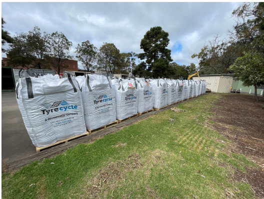
Recycled crumbed rubber used on Landy Field athletics track upgrade and resurfacing
